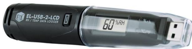
This standalone data logger measures and stores over 16,000 temperature and humidity readings from -35 to +80°C (-31 to +176°F) and 0 to 100%RH range at a resolution of 0.5°C (1°F) and 0.5%RH.
