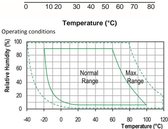
Long term exposure to humidity levels outside of the 'normal' range may temporarily offset RH measurements ( $\pm 3\%RH$  after 60 hours). Once returned to less extreme conditions the device will slowly return towards calibration state.
