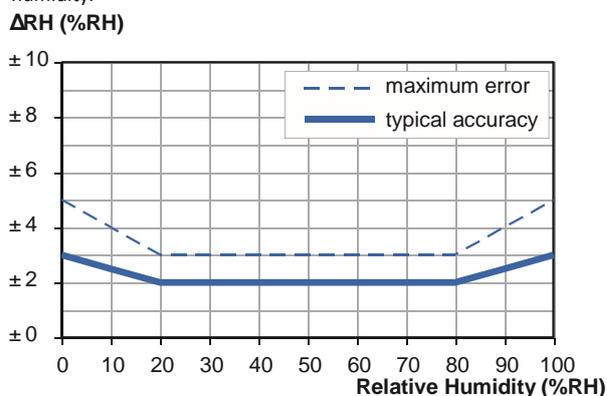
Typical accuracy of relative humidity measurements given in %RH for temperatures 0 to 80°C.
